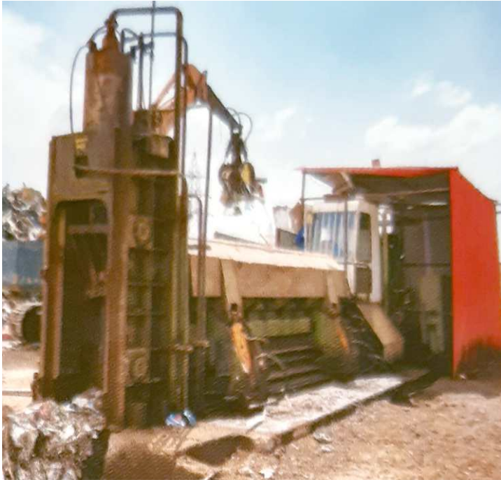
Heavy Duty Bailer Capacity of 350 kg to 500 kg per hour
